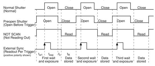
Figure 31. Timing Diagram for External Sync Mode (+ edge trigger)
